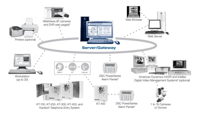
A variety of video products have been tested successfully using WebViews. For a complete list, contact Kantech sales Direct: using RS-232 or RS-485 with USB-485 or VC-485 converter, KT-100 using RS-485 with converter IP using Kantech IP Link or KT-400 Ethernet controller
